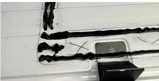
Abb. 2-6: Adhesive application on the roof
