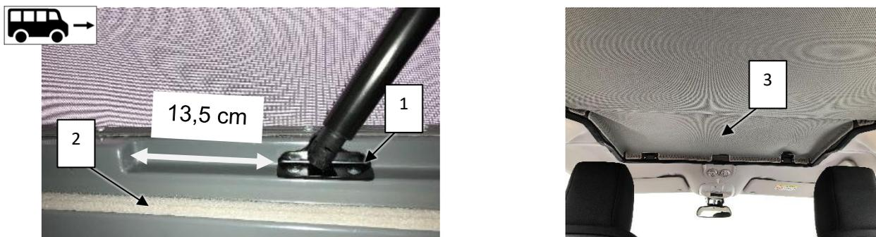
Fig. 9-1: Gas spring position and loop tape
