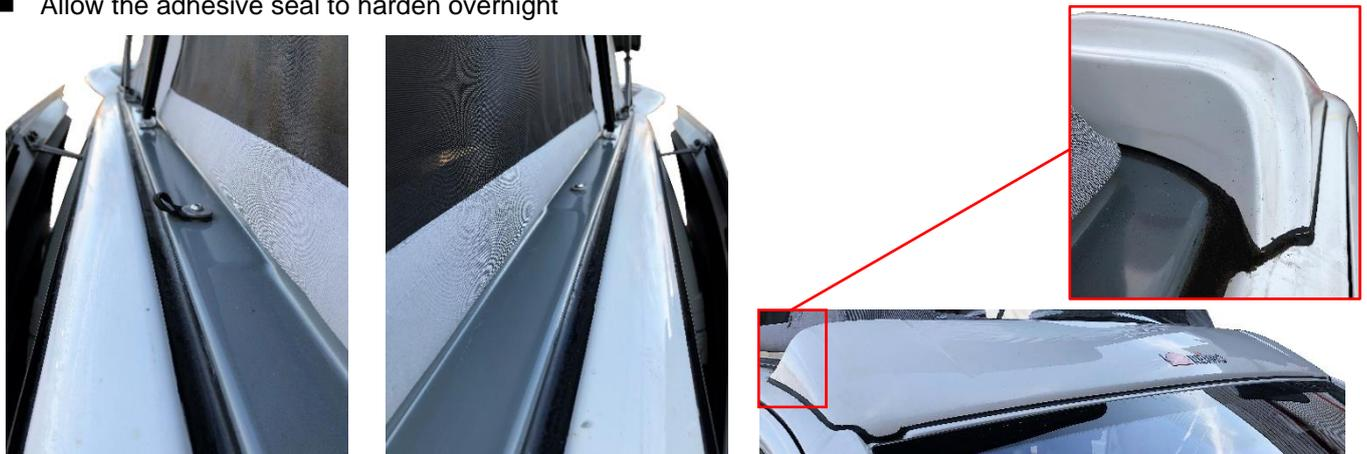
Fig. 7-1: Seaming of the EasyFit frame and the front spoiler
