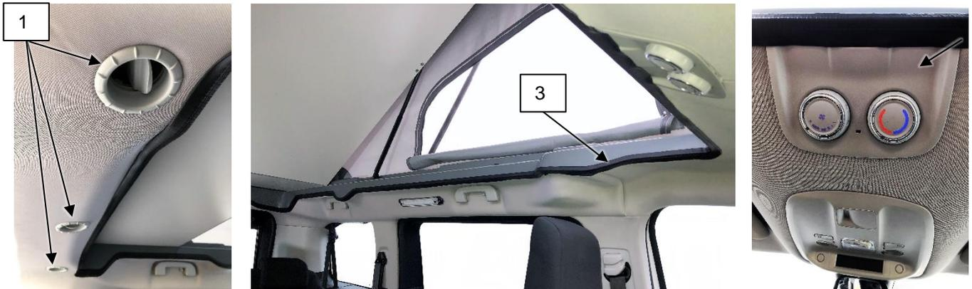
Fig. 10-4: Fitting the headlining
