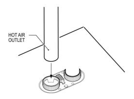
If fitting an under floor heater, fit the air duct into the hot air outlet fitting.
