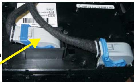
Connect the harness BLUE wire to the VIOLET-ORANGE (Pos. 55) wire in the 60-pin Grey-Light Blue connector at the back of the BCM.
