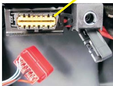
Remove the plastic cover from the 16-pin BLACK OBD connector under the BCM and connect the harness RED connector.
