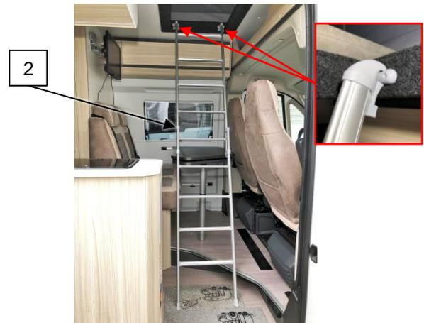
Abb. 9-1: Mounting the hooks in the vehicle
