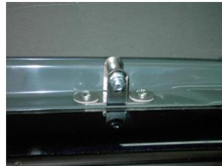
Fig. 1-1: Brackets of the pop top roof
