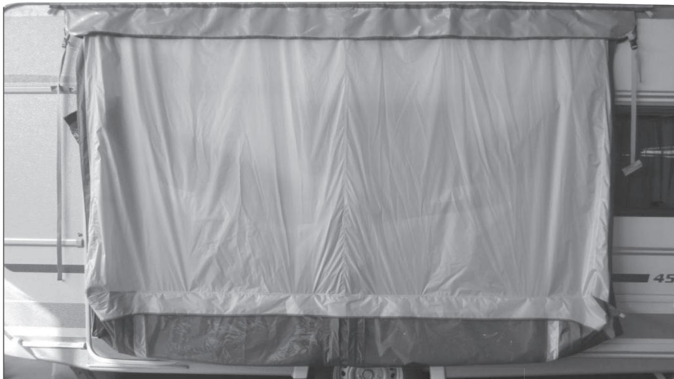
2. Lift up the front panel and secure in place with the buckle as attached picture.
