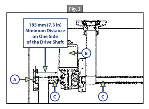
3. When cutting the drive shaft to measure, leave a minimum of 5 mm (0.21 in), maximum 10 mm (0.40 in), distance between each shaft and the motor (Fig. 4A).
