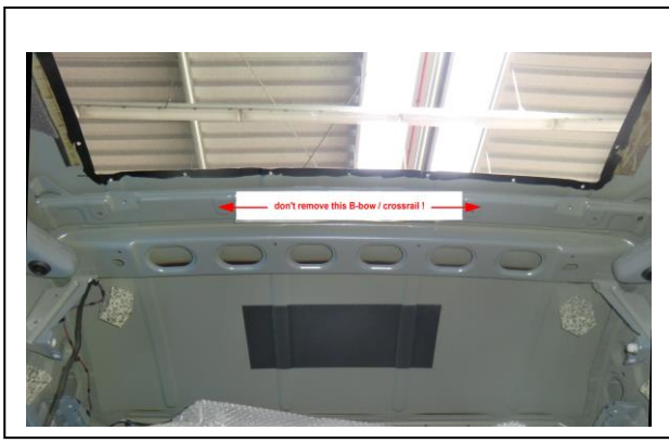
1. Cut our starts 30 mm behind end of B-Post
