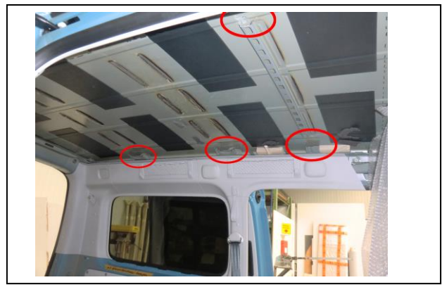
2. ends of cutted bows will be needed to fix frame
