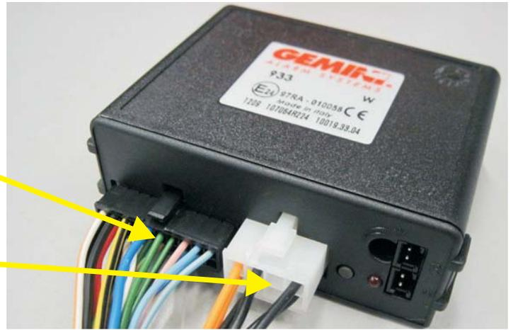
Plug the harness connectors into the alarm unit corresponding sockets.
