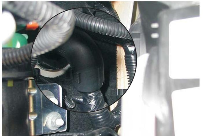
Run the siren and bonnet switch wires through the OE grommet behind the driver side headlight, over the ABS pump.
