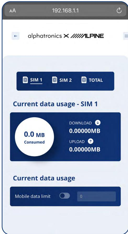
In this level, the data consumption of the respective SIM card can be determined and displayed.
