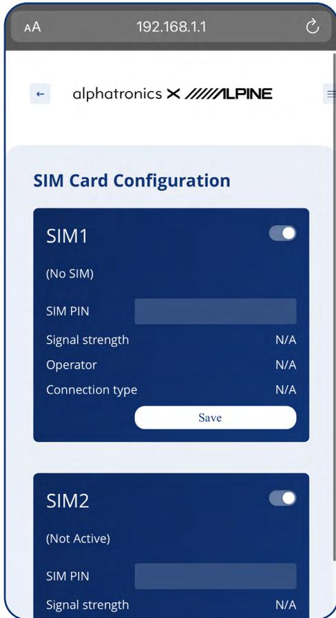
The most important information about the SIM cards can be viewed here. In addition, the SIM PIN of the corresponding card can be stored here.
