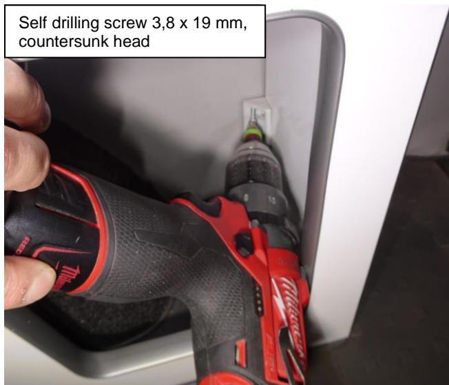
Body in correct position, screw positions
