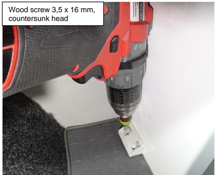
Screwing body into wheel housing
