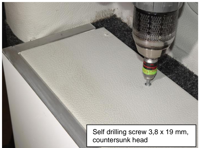
Screwing body into wheel housing
