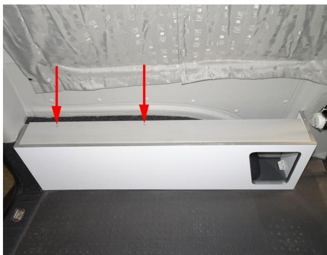
Body in correct position, screw positions
