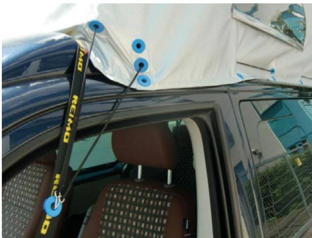
As needed you can pull the elastic strap from inside through the eyelet in the front corner. Then you can fix the strap at the eyelet of the front belts.
